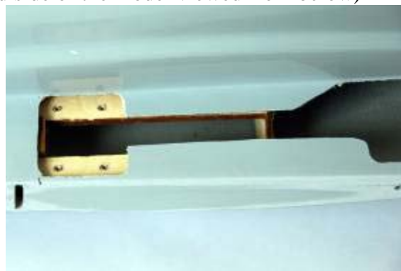
Mask the remaining area as shown above and in the template. (The cut out shown is from the right hand side of the model viewed from below)
